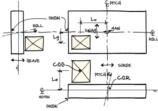
Figure 1: Position of cargo w.r.t. barge centre of rotation
