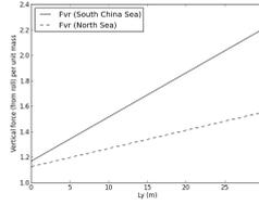
Figure 7: Effect of  $L_y$  on inertia forces
